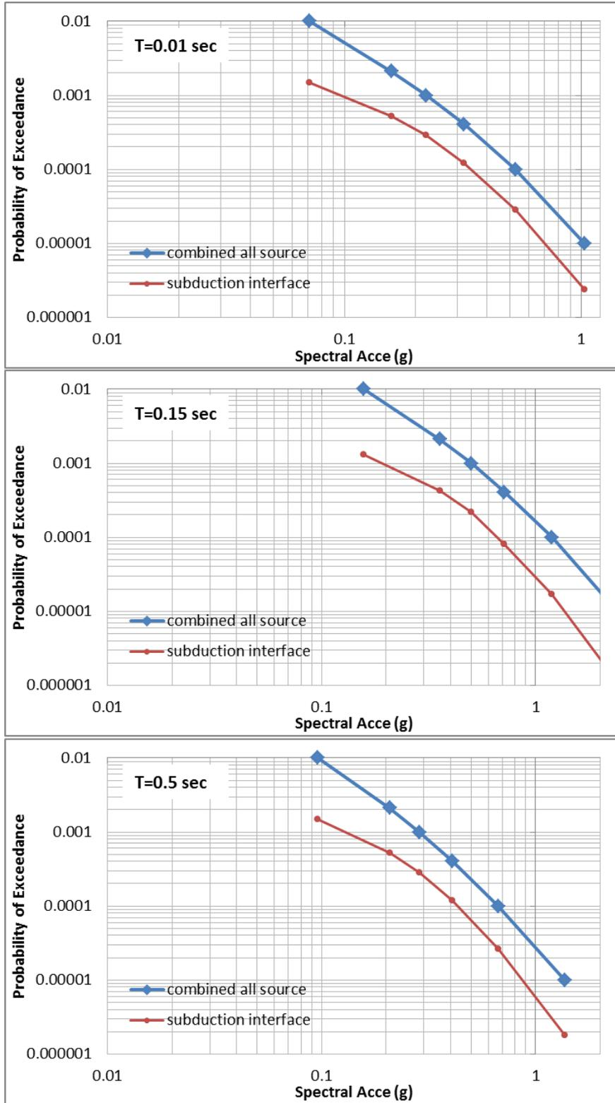
Figure 2 Seismic hazard spectra at AEP of 1/10,000 for subduction interface, crustal plus intra-slab earthquake sources, and all combined sources (UHRS)
