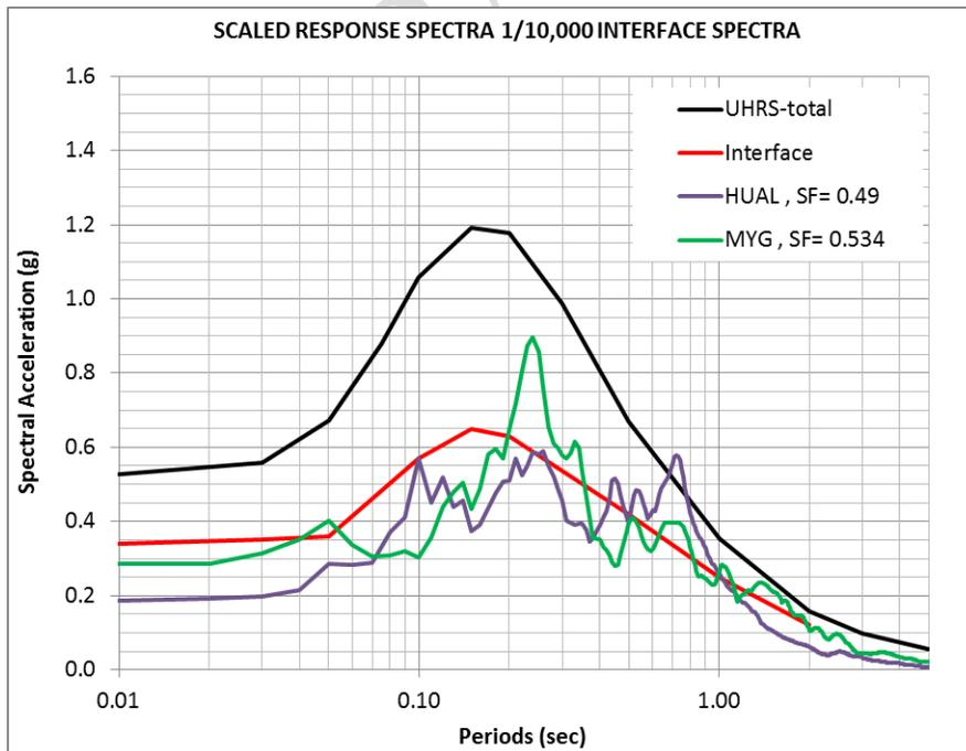
Figure 4 Response spectra for three crustal earthquake records scaled to fit 1/10,000 seismic hazard spectra for crustal plus intra-slab events
